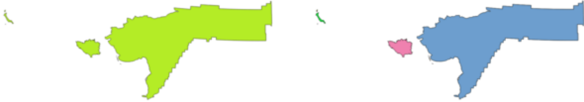
Рис. 23.54: Left the multipart source layer and right the single part output result
