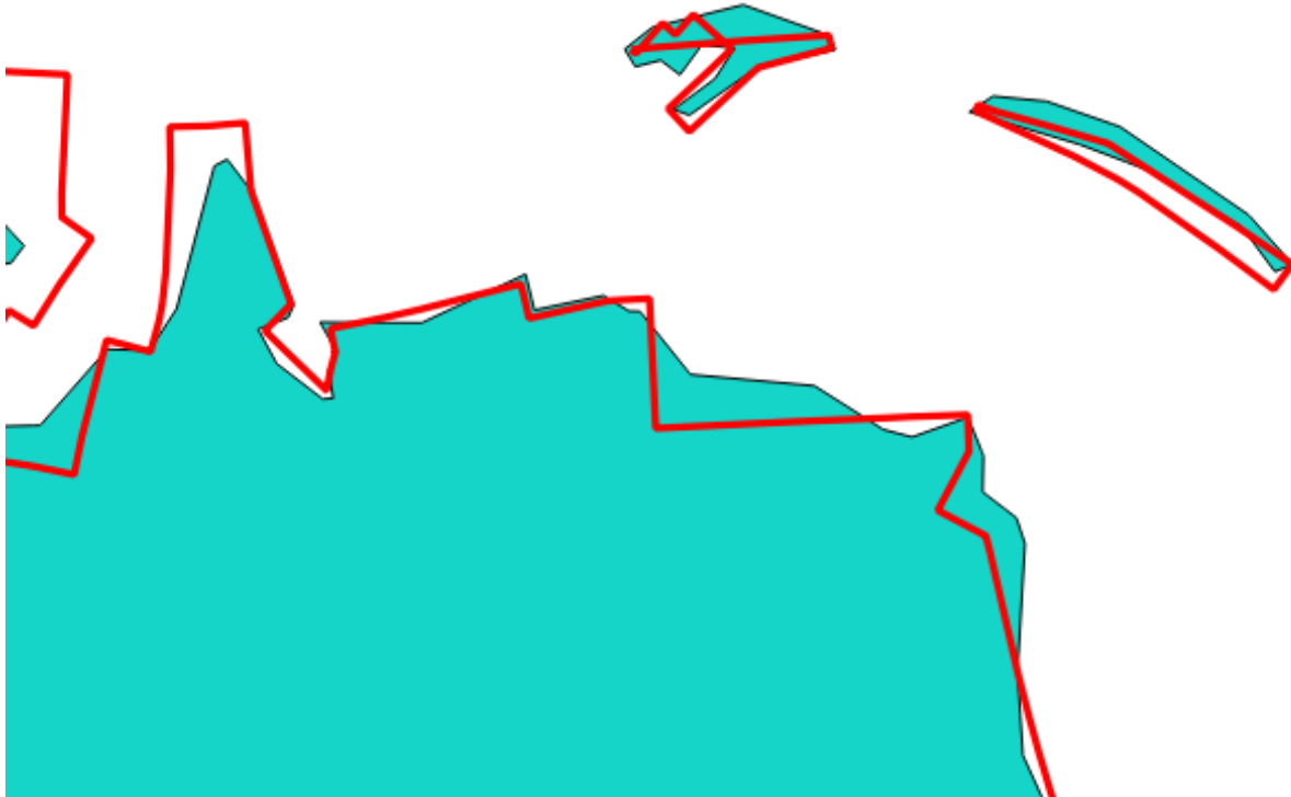
Fig. 23.57: In blue the source layer and in the red orthogonalized result
