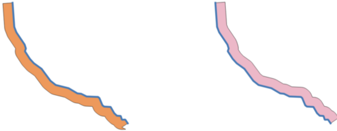
Fig. 23.66: Left versus right side buffer on the same vector line layer
