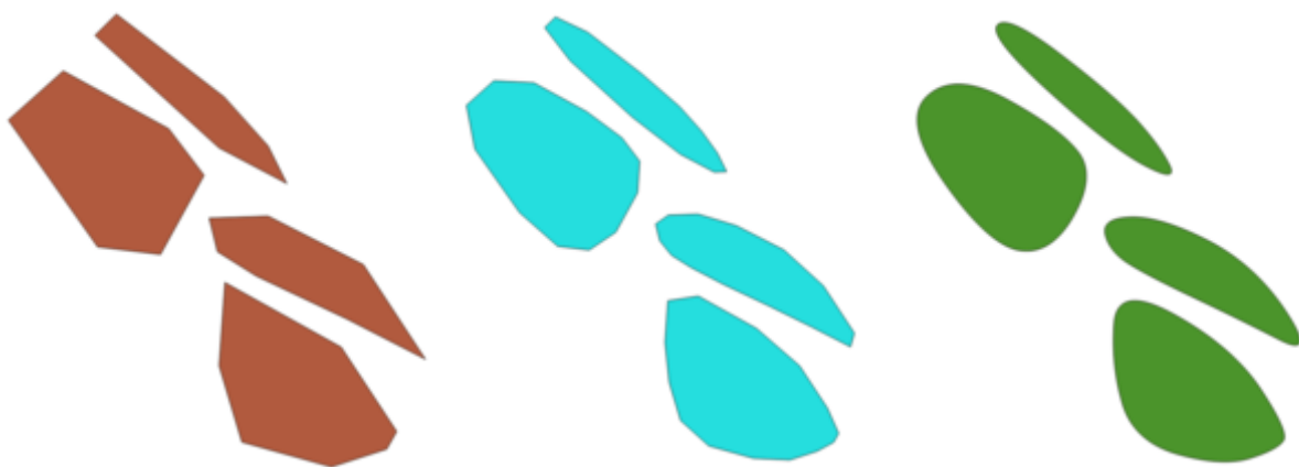
Fig. 23.67: Increasing number of iterations causes smoother geometries
