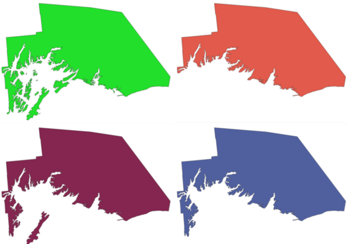
Fig. 23.49: Clockwise from top left: original multipart feature, one, two and three biggest parts kept
