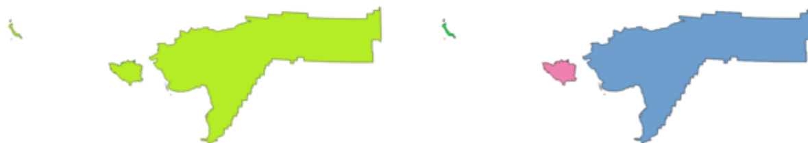
Abb. 23.54: Left the multipart source layer and right the single part output result
