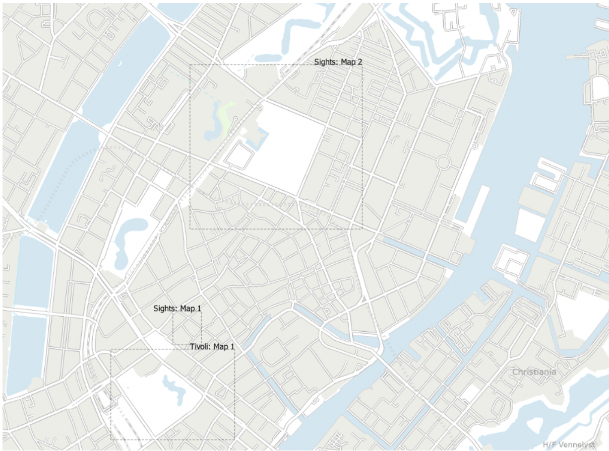
Abb. 11.13: Example of layout extents displayed in a QGIS project with two print layouts. The print layout named ‚Sights‘ contains two map items, while the other print layout contains one map item.
