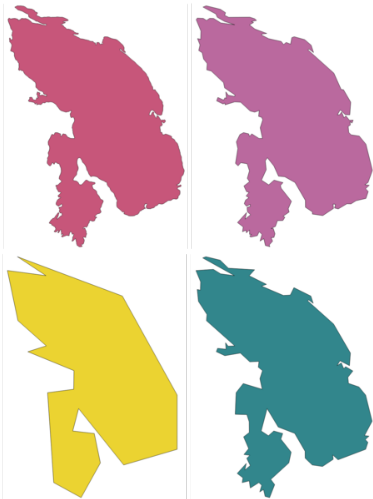
Obr. 23.65: Clockwise from top left: source layer and increasing simplification tolerances
