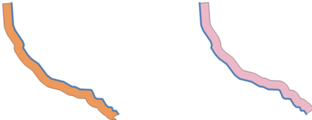
Obr. 23.66: Left versus right side buffer on the same vector line layer
