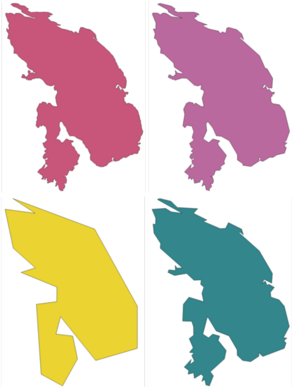
Fig. 23.65: Clockwise from top left: source layer and increasing simplification tolerances
